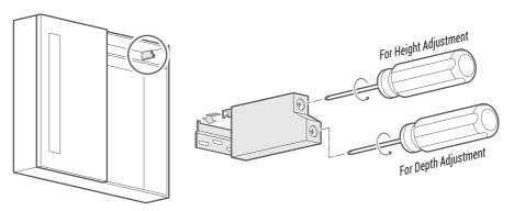
Adjustments can be made using the two screws on the cabinet hangers.
