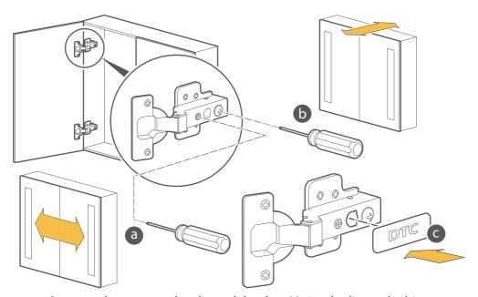
Once you have correctly adjusted the door(s) simply clip on the hinge cover **c**)
