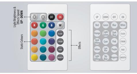
There are four **MODE** buttons giving the effects described in the table show below. To operate these simply point your remote towards the black sensor and select the required function and click **once**. The speed of the transitions can be increased or decreased by pressing the **UP** or **DOWN** buttons. Simply select a static colour to cancel the function.
